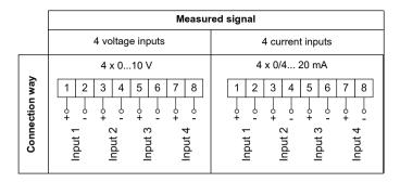
The polarization is optional when supplying by d.c. voltage.
