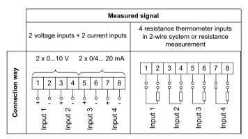
Fig. 4 connection way of input signals
