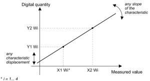
X1 Wi value in the module input of systems => Y1 W1 digital value
