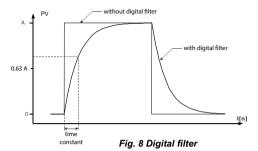
In the case where the measurement is unstable, you can enable the digital filter with a programmable time constant. You need to set the minimum filter time constant at which the measurement is stable. A high time constant can cause delays in reading the rapid changes in the measurement.
